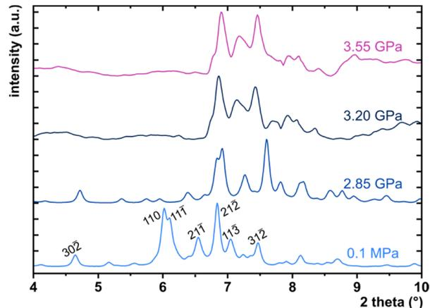
Fig. 11 PXRD collected for PTCDI-Ph phase II at 0.1 MPa, 2.85 and 3.20 GPa as well as phase III at 3.55 GPa. The measurements were performed using synchrotron X-ray diffraction ( $\lambda = 0.4099 \text{ \AA}$ ). Patterns for 0.1 MPa and 2.85 GPa are the calculated diffractograms from single-crystal measurements.
