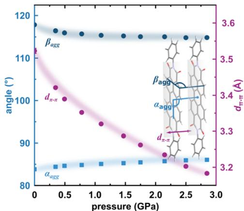
Fig. 7 Changes in the packing of PTCDI-Ph phase II under compression (b): purple circles mark the distance between  $\pi$ -stacked molecules ( $d_{\pi-\pi}$ ) and blue symbols represent the packing angles  $\alpha_{agg}$  and  $\beta_{agg}$  (cf. Fig. 4).
