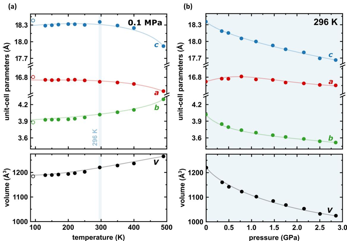
Fig. 3 Temperature (a) and pressure (b) dependence of the unit-cell dimensions *a*, *b*, *c* (top) and its volume (bottom) for PTCDI-Ph phase II. Open symbols mark the data previously reported by Sato and Mizuguchi.<sup>38</sup> The estimated standard deviations (ESDs) are smaller than plotted symbols. The blue highlight indicate the data measured at 296 K. The changes in monoclinic angle  $\beta$  are shown in Fig. S5 in the ESI†
