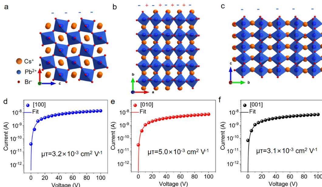
Fig. 2 (a–c) Arrangement of  $[\text{PbBr}_6]^{4-}$  octahedrons in the  $\text{CsPbBr}_3$  crystal structure, and (d–f) photocurrent fitting curves of the [100], [010], and [001] wafers of  $\text{CsPbBr}_3$  crystal.
