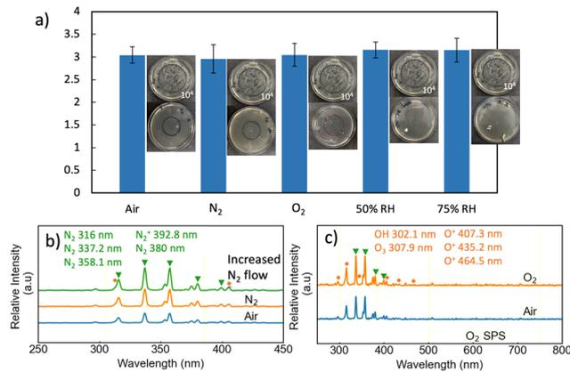
Fig. 3 (a) CD sterilization effectiveness of *E. coli* on N95 masks at different atmospheres; (b) spectrum generated by CD under N<sub>2</sub> flow; (c) spectrum generated by CD under O<sub>2</sub> flow.
