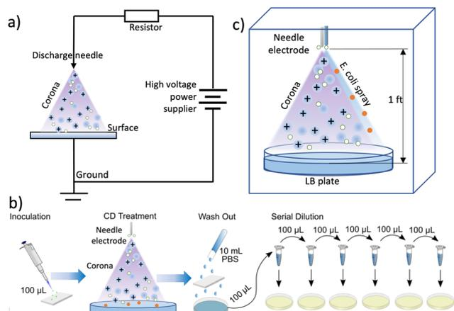
**Fig. 1** (a) Schematic of the CD treatment setup; (b) procedure of the sterilization experiments, including inoculation with microorganisms, CD treatment, washing out surviving colonies, serial dilution using PBS, and plating; (c) schematic of CD air sterilization test setup.
