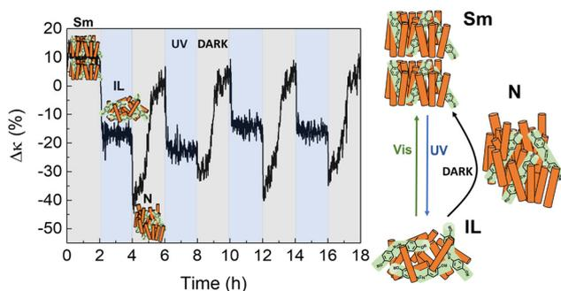
**Fig. 7** UV/Dark cycles of 8CB: azobenzene molecular system at  $\approx 290$  K. Three different thermal states can be identified in this case, associated with the different  $\kappa$  values of the Sm-LC, N-LC and IL, as observed in Fig. 5(b).
