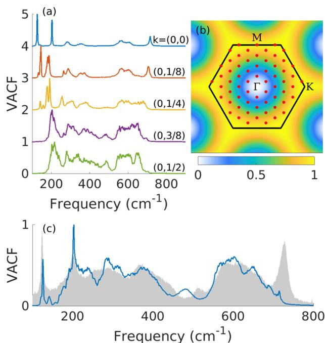
**Fig. 5** (a) Phonon density of states for wavevectors along the  $\Gamma$ - $M$  path. Labels on the right show the coordinates of the wavevector. (b) First Brillouin zone (black lines) with the  $8 \times 8$   $k$ -point mesh (red dots). The colormap represents the weights used in the phonon-projected VACF. (c) Weighted phonon-projected VACF. Modes outside  $\Gamma$  are weighted using the colormap of (b). The gray areas show the experimental Raman spectrum for comparison.
