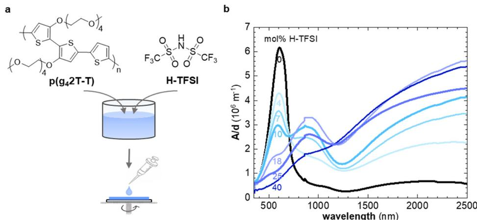
Fig. 1 (a) Molecular structures of p(g<sub>4</sub>2T-T) and H-TFSI and schematic of co-processing of polymer and dopant. (b) UV-Vis spectra of thin films of p(g<sub>4</sub>2T-T) co-processed with H-TFSI and aged for 2 days (mol% of H-TFSI calculated with respect to the number of thiophene rings).
