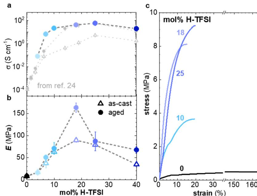
Fig. 6 (a) Electrical conductivity  $\sigma$  (top) of films of p( $g_4$ 2T-T) co-processed with H-TFSI and aged for 2 days (solid blue circles), as well as as-cast films (open grey triangles) and films aged for 3 days from ref. 24 (full grey circles). (b) Young's modulus  $E$  of as-cast samples (open triangles) and samples aged for 14 days (solid circles). (c) Stress–strain curves recorded at room temperature during tensile deformation of samples aged for 14 days.
