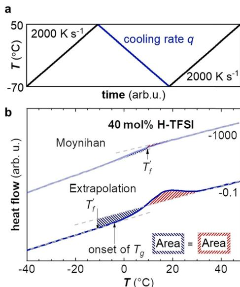
Fig. 4 (a) Fast scanning calorimetry (FSC) protocol: the sample is first heated to 50 °C, then cooled at rate  $q$  ranging from  $-0.1$  to  $-1000$  K s $^{-1}$ , and finally heated again at 2000 K s $^{-1}$ . (b) FSC heating thermograms after fast ( $q = -1000$  K s $^{-1}$ ; light blue) and slow ( $q = -0.1$  K s $^{-1}$ ; dark blue) cooling of p(g $_4$ 2T-T) co-processed with 40 mol% H-TFSI and aged for 2 days.
