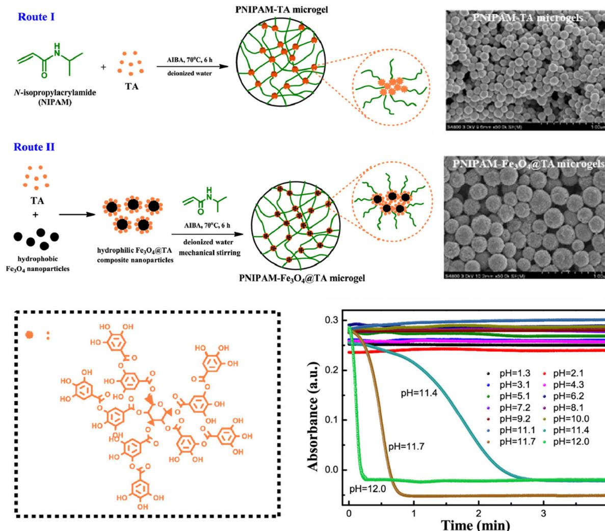
Fig. 6 PNIPAM–TA microgels fabricated *via* hydrogen bonding and the pH-dependent degradation. Reproduced with permission from ref. 102. Copyright 2019 American Chemical Society.
