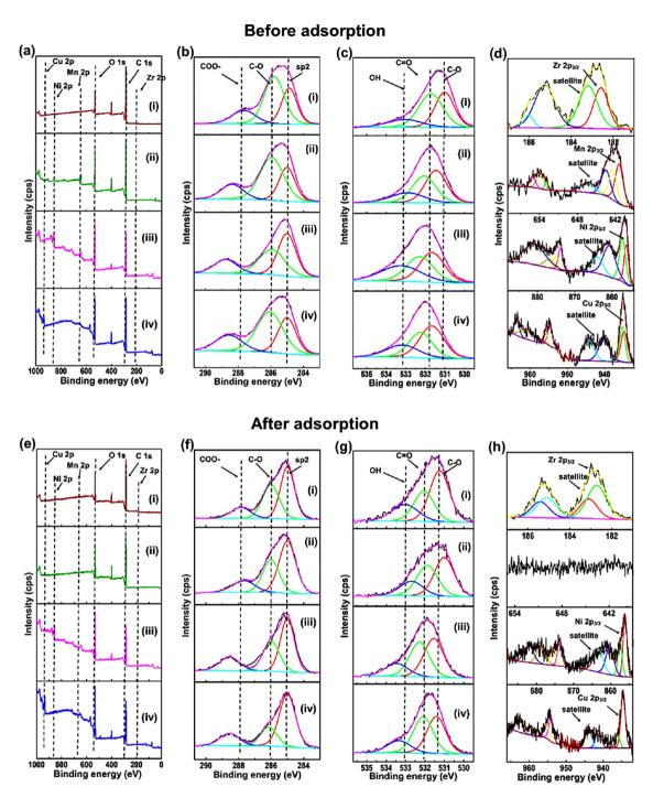
Fig. 6 XPS analysis of (i) Zr-BDC, (ii) Mn-BDC (iii) Ni-BDC and (iv) Cu-BDC before and after glucose adsorption: (a and e) survey spectra; high-resolution XPS spectra for (b and f) C 1s, (c and q) O 1s, and (d and h) M 2p (where M = Zr, Mn, Ni, and Cu).
