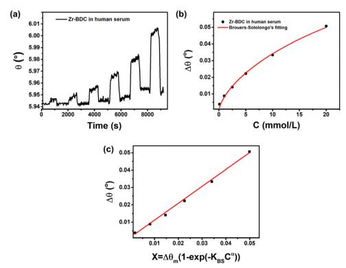
Fig. 8 (a) SPR dynamic response, (b) the Brouers-Sotolongo isotherm adsorption model fitting, and (c) the calibration curve of the hierarchical plate-like Zr-BDC to 0.1-20 mmol L<sup>-1</sup> glucose in a human serum/PBS solution.
