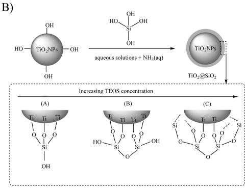
Fig. 2 (A) Hydrolysis and (B) condensation reactions of tetraethoxysilane (TEOS). Adapted with permission from ref. 22. Royal Society of Chemistry.
