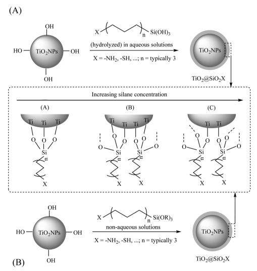
Fig. 3 The interaction between a general silane coupling agent and TiO<sub>2</sub>NPs in aqueous (A) and non-aqueous (B) solutions. Adapted with permission from ref. 22. Royal Society of Chemistry
