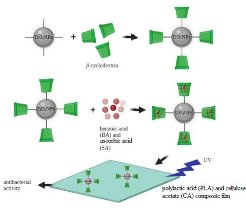
Fig. 5 β-Cyclodextrin-modified TiO<sub>2</sub>NPs for antibacterial applications. Adapted with permission from ref. 129. Copyright 2022 Elsevier.
