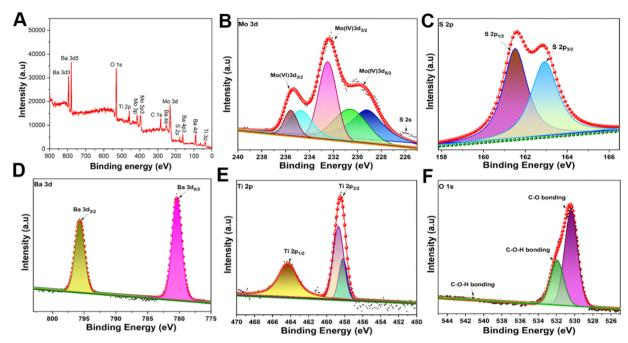
Fig. 2 High-resolution XPS spectra of MoS<sub>2</sub>@BT CSNPs. (A) MoS<sub>2</sub>@BT CSNPs survey spectrum, (B) spectra for the Mo 3d and S 2s of MoS<sub>2</sub>, (C) spectra for the S 2p orbits of MoS<sub>2</sub>, (D) spectra for the Ba 3d of BT, (E) spectra for the Ti 2p of BT and (F) spectra for the O 1s of BT.
