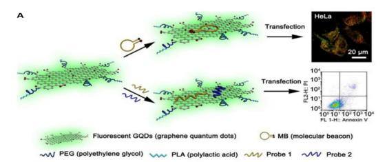
Fig. 4 Schematic illustration of (A) DNA/RNA co delivery by GQDs for cancer treatment.<sup>115</sup> Reprinted with permission from ref. 115.
