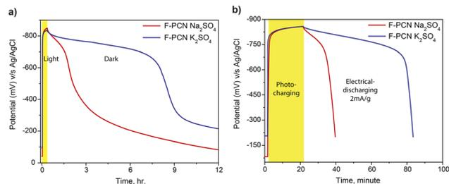
**Fig. 4** (a) OCP measurement on F-PCN in the presence of different electrolytes ( $M_2SO_4$  and 4-MBA) (b) Photo charging of F-PCN in the presence of different electrolytes for 20 minute (OCP) and subsequently electrical discharging with  $2 \text{ mA g}^{-1}$ . All the measurements are done in an inert condition.
