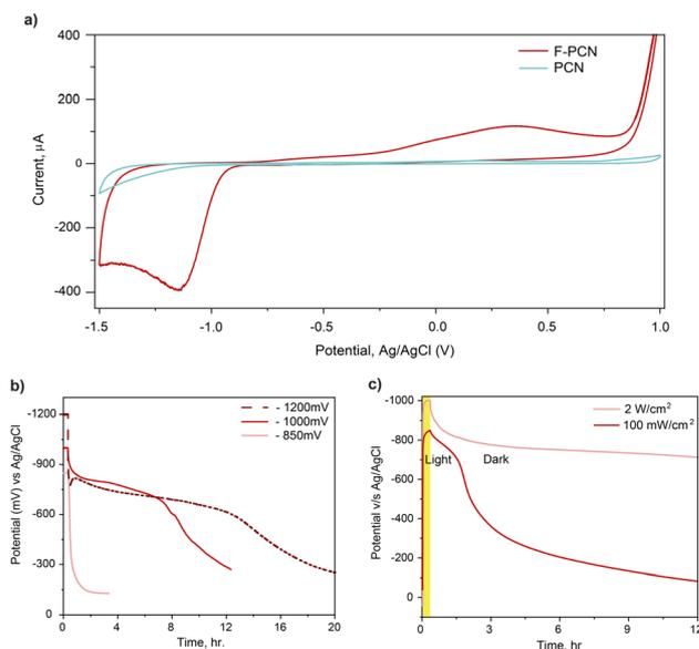
Fig. 2 (a) Cyclic voltammetry curve for PCN and F-PCN in 0.1 M Na<sub>2</sub>SO<sub>4</sub> and 5 mM 4-MBA, scan rate 5 mV s<sup>-1</sup> (b) charging F-PCN for 20 min with three different external biases in Na<sub>2</sub>SO<sub>4</sub> and 4-MBA electrolyte (c) charging F-PCN in Na<sub>2</sub>SO<sub>4</sub> and 4-MBA with different intensity lamp (1.5 AM). All the measurements are done under inert conditions.
