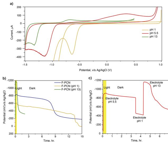
**Fig. 5** (a) Cyclic voltammetry on F-PCN at different pH of the electrolyte ( $M_2SO_4$  and 4-MBA) (b) OCP measurement of F-PCN at different pH of the electrolyte ( $M_2SO_4$  and 4-MBA) (c) OCP measurement on F-PCN, pH of electrolyte changed from 5.5 to 1 after 3 h of dark and again the pH to 13 after 4 h of dark.
