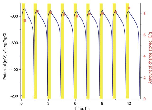
Fig. 6 F-PCN cyclability (multiple time 20 minute photo-charging and subsequently electrical discharging with a current density of  $2 \text{ mA g}^{-1}$ ) using  $0.1 \text{ M K}_2\text{SO}_4$  and  $5 \text{ mM 4-MBA}$  electrolyte.
