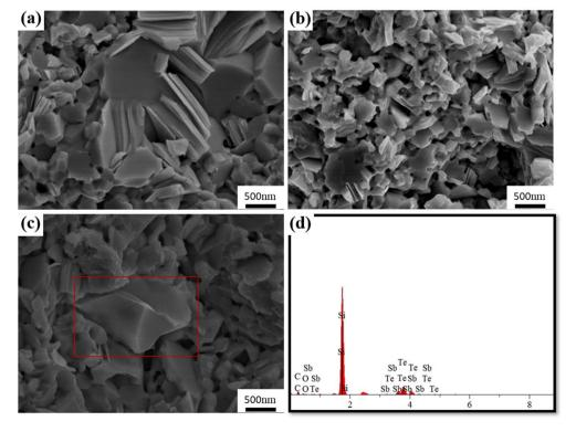
Fig. 3 Fracture morphologies and EDS compositions of  $Bi_{0.5}Sb_{1.5}Te_3/xvol\%$  SiC (x=0,0.6) bulk samples. Fracture morphologies of (a) x=0 and (b) and (c) x = 0.6 samples; (d) EDS composition of the rectangular area in (c).
