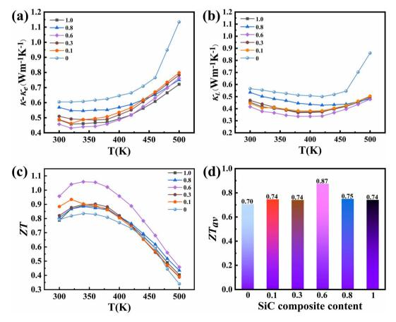
Fig. 6 (a) The combined lattice and bipolar thermal conductivity, (b) lattice thermal conductivity, and (c) ZT values as a function of temperature for  $Bi_{0.5}Sb_{1.5}Te_3/x$  vol% SiC (x = 0, 0.1, 0.3, 0.6, 0.8,and 1.0) composite samples. (d) Average ZT values at 300–500 K for the composites.
