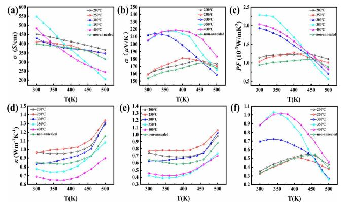
Fig. 1 Temperature-dependent thermoelectric properties of  $Bi_{0.5}Sb_{1.5}Te_3$  materials under different heat treatment conditions: (a) electrical conductivity, (b) Seebeck coefficient, (c) power factor, (d) thermal conductivity, (e) the combined lattice and bipolar thermal conductivity, and (f) ZT values.
