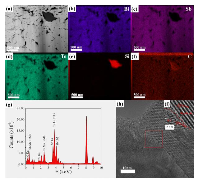
Fig. 4 (a) The microstructure of  $Bi_{0.5}Sb_{1.5}Te_3/xvol\%$  SiC (x=0.6), (b-f) the distribution of Si, Bi, Sb and Te elements, (g) EDS composition of  $Bi_{0.5}Sb_{1.5}Te_3/xvol\%$  SiC (x=0.6), (h) high-resolution TEM images of x=0.6 samples, and (i) high-resolution TEM images of x=0.6 sample interfaces ((i) is the image of the red rectangular area in (h)).
