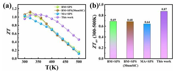
Fig. 7 Comparison of (a) temperature dependent ZT values and (b) ZT<sub>av</sub> for Bi<sub>0.5</sub>Sb<sub>1.5</sub>Te<sub>3</sub>/SiC composites prepared by different methods.
