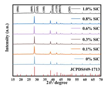
Fig. 2 XRD patterns of  $Bi_{0.5}Sb_{1.5}Te_3/x$  vol% SiC (x = 0, 0.1, 0.3, 0.6, 0.8,1.0) pellet samples after heat treatment.
