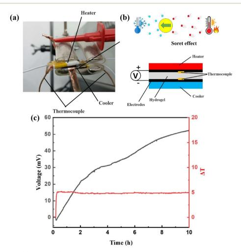
Fig. 8 Schematic diagram of (a) device and (b) principle for testing the thermoelectric effect of APC-PVA@ZnCl<sub>2</sub> materials. (c) The relationship of the change in potential of the APC-PVA@ZnCl<sub>2</sub> material with the change in temperature and time.
