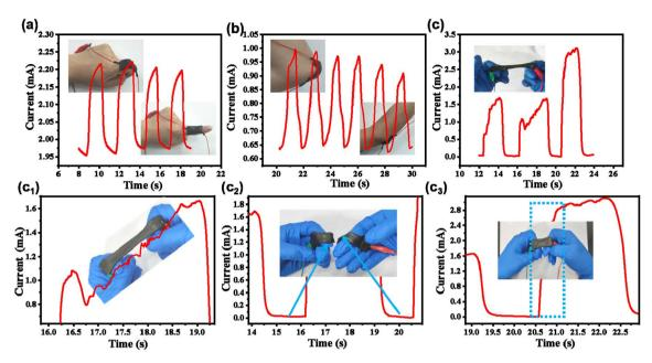
Fig. 5 Monitoring the changes of electrical signals during (a) finger and (b) elbow movements and  $(c-c_3)$  material stretching under different tensile conditions based on the APC-PVA@ZnCl<sub>2</sub> sensor.
