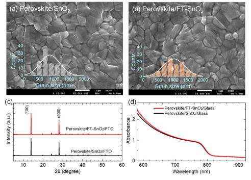
Fig. 3 Top-view SEM image of the perovskite layer coated on (a) bare  $SnO_2$  and (b) FT- $SnO_2$ . Insets show grain size distribution. (c) XRD patterns of the perovskite films formed on  $SnO_2$ - and FT- $SnO_2$ -coated FTO substrate. (d) Absorbance of the perovskite films deposited on  $SnO_2$ - and FT- $SnO_2$ -coated glass substrate.
