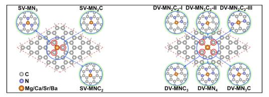
Fig. 1 Schematic illustrations of the AE-SAC systems with single Mg/Ca/Sr/Ba atom anchoring on the graphene support with different coordination environments.
