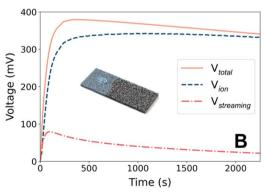
Fig. 2 (A). Comparison of the experimental voltage profile (black dots) and the model prediction (orange line). In the experiment, a 0.3 mL water droplet was placed on the left side of the carbon black-coated cotton fabric (inset). (B.) Voltage (defined as the potential difference between the head and tail ends of the substrate) predicted from the model (orange) and its decomposition into contributions from ions (navy) and streaming (red).
