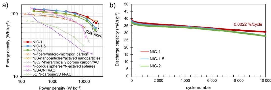
Fig. 7 (a) Ragone plot showing the energy/power performance of the NICs and (b) long-term cycling test performed at 2 A g<sup>-1</sup>.
