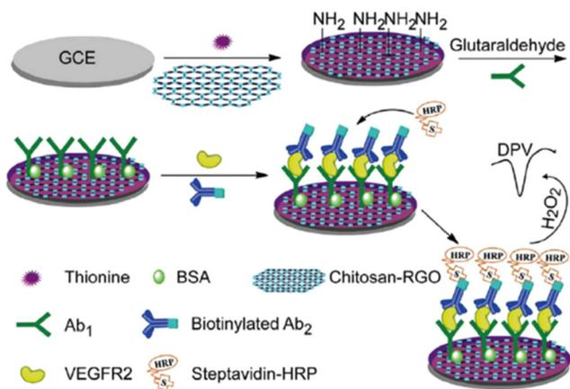
**Fig. 5** Electrochemical detection of vascular endothelial growth factor receptor 2 (VEGFR2) in the presence of a chitosan-rGO based GCE. Reproduced from ref. 111 with permission from Elsevier, copyright [2017].
