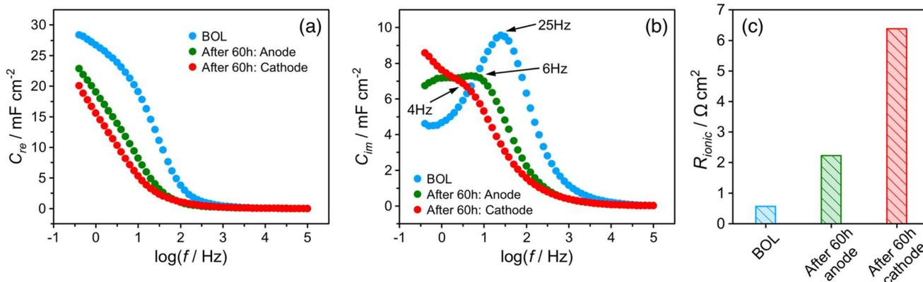
Fig. 3 Experimental (a) real and (b) imaginary capacitance plots of the catalyst layer at the BOL, anode, and cathode after a 60 hour stability test. (c) Corresponding calculated ionic resistance in the catalyst layer.
