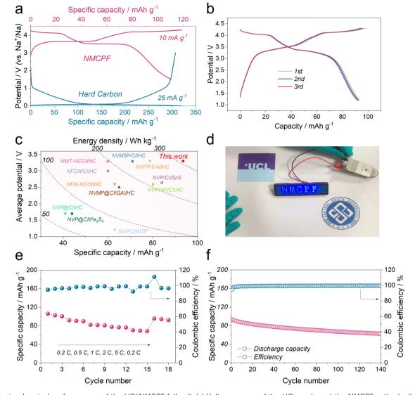
Fig. 5 Electrochemical performances of the HC||NMCPF full cell. (a) Voltage curves of the HC anode and the NMCPF cathode. (b) Chargedischarge profiles of the HC||NMCPF full cell for the initial three cycles at 0.5C ( $1C = 110 \text{ mA g}^{-1}$ ). (c) Comparison of our work with previous reported works. (d) Picture of a LED badge powered by the HC||NMCPF full cell. (e) Rate capability of the full cell. (f) Cycling stability of the full cell at 0.5C.
