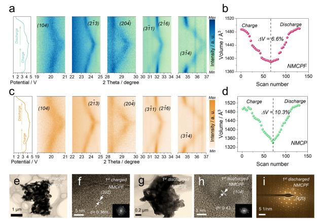
Fig. 3 Structural evolution. (a, b) *In situ* XRD contour patterns and corresponding changes of the lattice volume of NMCPF. (c, d) *In situ* XRD contour patterns and corresponding changes of the lattice volume of NMCP. (e, f) TEM and HRTEM images (inset: FFT pattern) of the 1<sup>st</sup> charged NMCPF. (g–i) TEM, HRTEM images (inset: FFT pattern) and the SAED pattern of the 1<sup>st</sup> discharged NMCPF.
