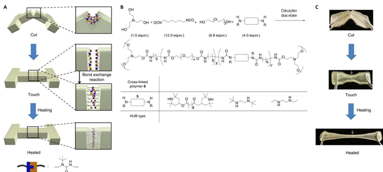
Fig. 7 Preparation and self-healing of a crosslinked poly(urethane-urea) gel with hindered urea bonds. (A) Illustration of the self-healing process *via* bond exchange. (B) Synthetic route to generate the polymer. (C) Selected snapshots during the self-healing experiment of poly(urethane-urea). The arrow indicates the cut position. Adapted from ref. 53 with permission from Springer Nature, copyright 2014.
