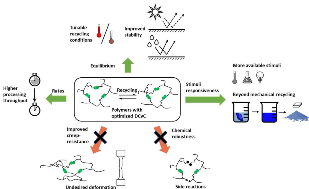
Fig. 4 Achievable improvements in recyclable dynamic networks *via* recycling-by-design strategy. Optimized DCVC-containing polymeric materials can exhibit tunable recycling conditions, fast (re)processing, various recycling approaches, and improved stability against side reactions or undesirable deformation.
