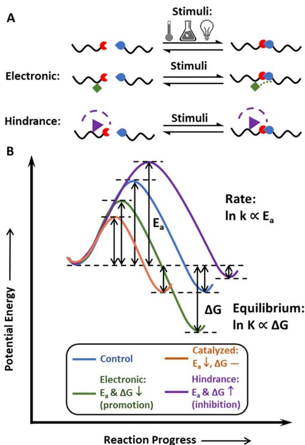
Fig. 2 (A) Generic dynamic covalent chemistry scheme related to equilibrium control through electronic/steric effects. (B) Control of reaction equilibrium and rate (rate constant:  $k$ ) via steric hindrance and electronic effects. Blue: control. Orange: catalyzed. Green: electronic effects (promote the reaction in this case). Purple: steric effects (inhibit the reaction in the case shown in (A)).
