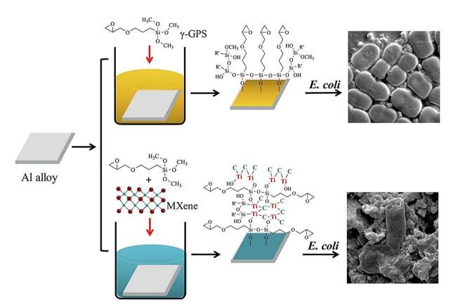
Fig. 6 MXene-hybridized silane films with antibacterial properties; MXene ( $Ti_3C_2$ ) sheets were hybridized into the  $\gamma$ -glycidoxypropyltrimethoxysilane (γ-GPS) film on AA2024 aluminum (Al) alloy surface. Reproduced with permission from ref. 27 Copyright 2020 Elsevier.
