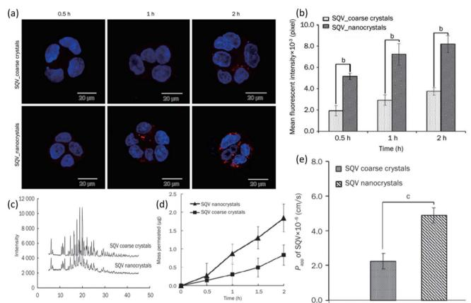
Fig. 11 (a) Cellular uptake of SQV coarse and nanocrystals was observed *via* laser scanning microscope. (b) The fluorescence intensity of cells was analyzed quantitatively. (c) XRPD diffraction pattern of SQV coarse and nanocrystals. (d) Permeation profiles of SQV through a monolayer of Caco-2 cells and (f) permeability coefficient of SQV across monolayers (reprinted with permission from ref. 106 Copyrights 2015 Nature).
