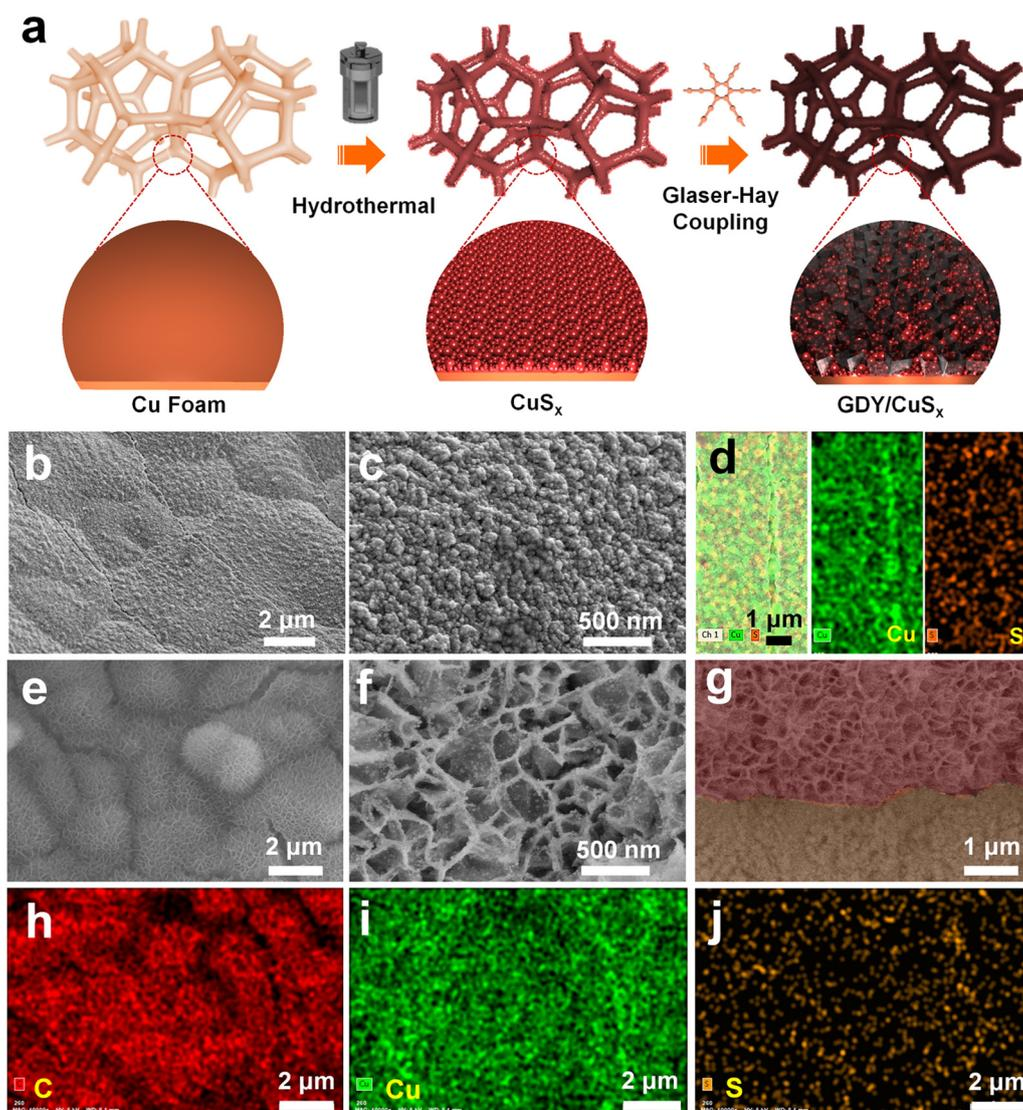
**Fig. 1** (a) Schematic representation of the synthesis route of GDY/CuS<sub>x</sub>; and (b) low- and (c) high-magnification SEM images of CuS<sub>x</sub>. (d) Energy dispersive spectroscopy mapping of CuS<sub>x</sub>. (e) Low- and (f) high-magnification SEM images of GDY/CuS<sub>x</sub>. (g) Cross-section SEM image of GDY/CuS<sub>x</sub>; and (h, i and j) energy dispersive spectroscopy mapping of GDY/CuS<sub>x</sub>.
