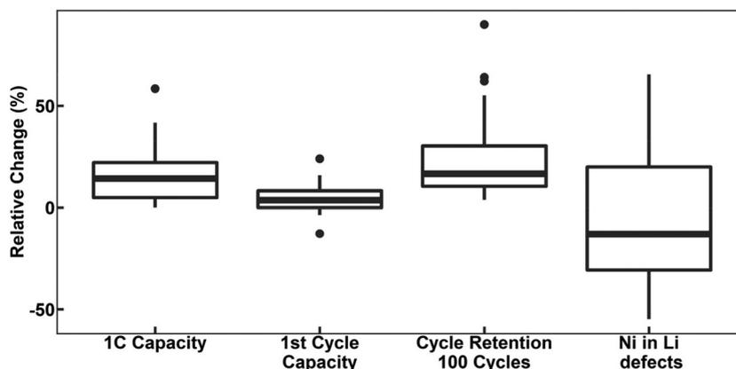
Fig. 7 Box-and-whisker plot of the relative change of 1C capacity ( $n = 16$ ), first-cycle capacity ( $n = 22$ ), capacity retention after 100 cycles ( $n = 22$ ), and  $\text{Ni}_{\text{Li}}^{\bullet}$  defects ( $n = 11$ ) of Nb-doped LTMOs applied for LIBs.
