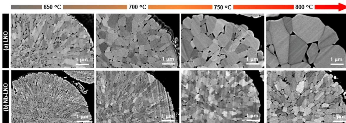
Fig. 9 Cross-sectional SEM images of (a) as-prepared LNO and (b) Nb-LNO calcined at 650–800 °C. Adapted from ref. 115. Copyright 2023, Wiley-VCH GmbH.
