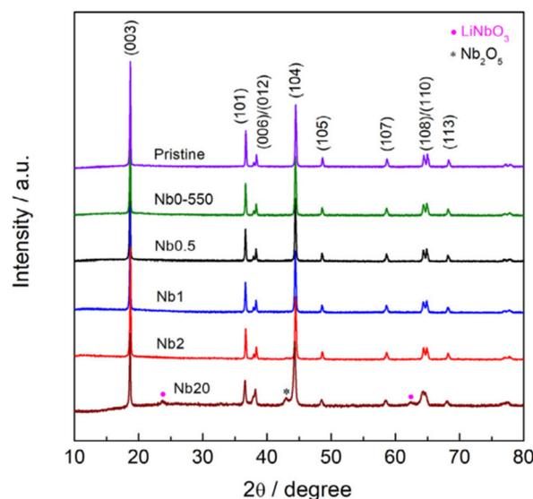
**Fig. 4** XRD patterns of NCM622 coated with different loadings (wt%) of LiNbO<sub>3</sub> prepared from an ammonium niobium oxalate sol-gel method. Reproduced with permission from ref. 56. Copyright 2021, Elsevier.
