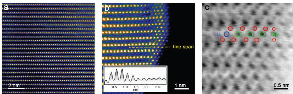
**Fig. 8** STEM images of Nb-doped  $\text{Li}_{1.2}\text{Mn}_{0.54}\text{Ni}_{0.13}\text{Co}_{0.13}\text{O}_2$ . (a) HAADF image of the bulk. (b) HAADF image of the surface near region. (c) ABF-enlarged image of the surface shown in panel (b). Adapted from ref. 137. Copyright 2018, Wiley-VCH GmbH.
