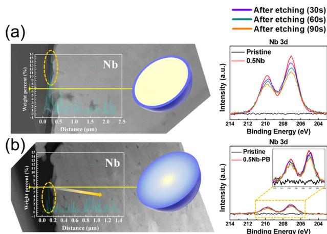
**Fig. 2** Cross-sectional scanning TEM (STEM) with EDS line profiles of Nb across the yellow line for LiNi<sub>0.82</sub>Co<sub>0.12</sub>Mn<sub>0.06</sub>O<sub>2</sub>. Shown to the right is the corresponding material's Nb 3d XPS spectra with different etch times. Panel (a) refers to a coating methodology of introducing Nb, while panel (b) refers to a route of including Nb with the precursor reagents. Adapted from ref. 87. Copyright 2021, American Chemical Society.
