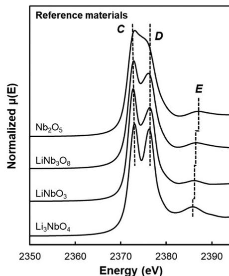
**Fig. 3** XAS of the Nb L<sub>3</sub>-edge of reference materials with Nb<sup>5+</sup> oxidation state. Dotted lines C and D correspond to LiNbO<sub>3</sub> peak position, while dotted line E is peak position of each reference material. Reproduced with permission from ref. 57. Copyright 2023, American Chemical Society.
