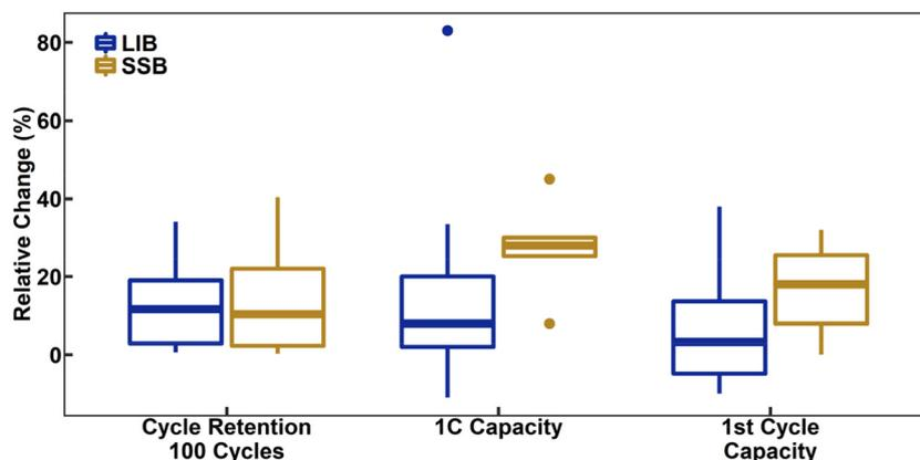
**Fig. 5** Box-and-whisker plot of the relative change of capacity retention after 100 cycles, 1C capacity, and first-cycle capacity of LiNbO<sub>3</sub> coatings with respect to "bare" NCM CAMs for both LIB and SSB systems. For cycle retention, *n* = 19 and 9 for LIB and SSB, respectively. For 1C capacity, *n* = 17 and 6 for LIB and SSB, respectively. For first-cycle capacity, *n* = 18 and 11 for LIB and SSB, respectively.
