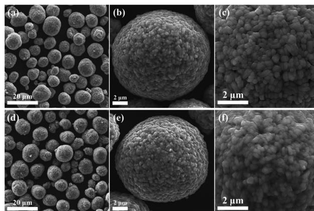
**Fig. 1** (a–c) SEM images of a pristine  $\text{LiNi}_{0.6}\text{Co}_{0.2}\text{Mn}_{0.2}\text{O}_2$  (NCM622) sample. (d–f) SEM images of coated NCM622 prepared from a ball-milling method with  $\text{Nb}_2\text{O}_5$  (0.5 mol%). Reproduced with permission from ref. 76. Copyright 2021, Elsevier.
