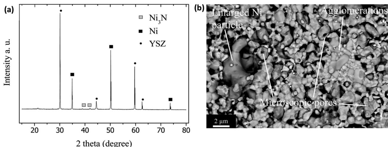
Fig. 5 (a) XRD pattern of Ni film on a YSZ disk after exposure to ammonia ( $100 \text{ mL min}^{-1}$ ) at 600 °C for 1 h. Reproduced with permission.<sup>36</sup> Copyright 2015, American Chemical Society. (b) SEM image of the anode surface at the fuel inlet region. Reproduced with permission.<sup>56</sup> Copyright 2019, Elsevier.
