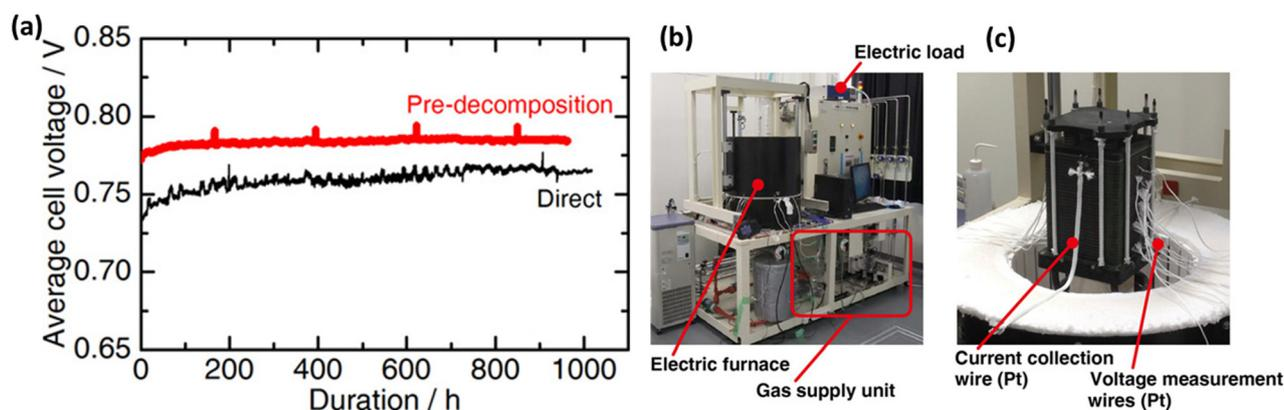
**Fig. 9** (a) Average cell voltage during a 1000 h durability test with ammonia fuel at 700 °C, 0.316 A cm<sup>-2</sup> current density, the photograph of (b) the stack evaluation system and (c) the 30-cell SOFC stack. Reproduced with permission.<sup>58</sup> Copyright 2020, Wiley-VCH.
