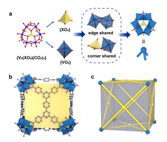
Fig. 2 (a) Structure of  $\{V_6(XO_4)(CO_2)_3\}$  (X = S/V) and the coordination mode. The six edge-sharing  $\{VO_6\}$  octahedra share the  $\{XO_4\}$  tetrahedral vertices to form the "3-pyramidal" MBB. (b) Structures of VMOC-6 and VMOC-7. (c) The simplified cubic model, with the yellow part of H₄PBPTA simplified to "4-planar" and the blue part of the hexanuclear vanadium cluster simplified to "3-pyramidal".
