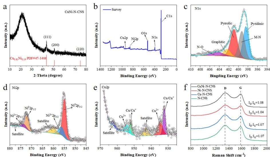
**Fig. 2** (a) X-ray diffraction patterns of CuNi-N-CNS. (b) The survey XPS spectrum of CuNi-N-CNS. (c–e) High-resolution spectra of N1s, Ni2p, and Cu2p of CuNi-N-CNS. (f) Raman spectra of CuNi-N-CNS, Ni-N-CNS, Cu-N-CNS, and N-CNS samples.
