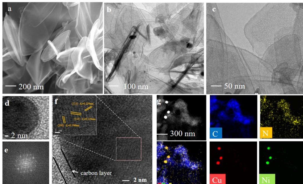
**Fig. 1** (a) High-resolution SEM patterns of CuNi-N-CNS. (b–c) TEM images of CuNi-N-CNS at different resolutions, and (d) CuNi@C in CuNi-N-CNS. (e) Corresponding FFT patterns. (f) HRTEM image and the enlarged image (g) EDS mapping of C, N, Cu, and Ni elements.
