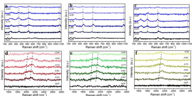
**Fig. 4** *In situ* Raman spectra of CO<sub>2</sub>RR over (a and d) T-Cu<sub>2</sub>O/Cu, (b and e) F-Cu<sub>2</sub>O/Cu and (c and f) O-Cu<sub>2</sub>O/Cu as a function of the applied potentials.
