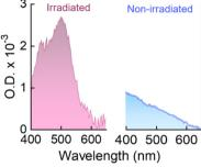
Fig. 4 Detection of iron ions. (A) Scheme of the purification process and the metal complex used for detecting the presence of released iron ions. Irradiated NFs (or non-irradiated for control) were filtered, and the filtrate was treated with 1,10-Phenanthroline (phen), resulting in the orange-red metal complex [Fe(phen)<sub>3</sub>]<sup>2+</sup>. (B) Extinction spectra obtained from the filtrates of NF dispersions without (blue) and with (magenta) 808 nm irradiation (P = 200 mW).
