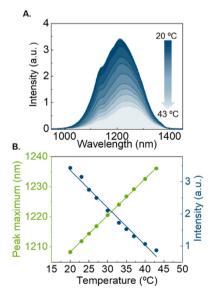
Fig. 1 Characterization of NIR Ag<sub>2</sub>S nanoparticles as LNThs. (A) Emission spectra of Ag<sub>2</sub>S LNThs obtained at different temperatures (from 20 to 43 °C). (B) Multiparametric thermal readouts of the emission spectra of Ag<sub>2</sub>S LNThs. Intensity and shifting of the peak maximum give inverse linear tendencies with Pearson correlation coefficients close to -1 for the emission intensity and 1 for the displacement.
