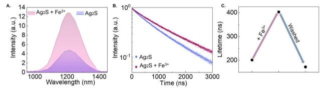
Fig. 5 Effect of iron ions. (A) Emission spectra measured at 20 °C of  $Ag_2S$  LNThs as synthesized and upon 2  $\mu$ L of 1 mM FeCl<sub>3</sub> addition. (B) Lifetime measurements measured at 20 °C of  $Ag_2S$  LNThs as synthesized and upon 2  $\mu$ L of 1 mM FeCl<sub>3</sub> addition. (C) Lifetime values measured at 20 °C of  $Ag_2S$  LNThs as synthesized, upon 2  $\mu$ L of 1 mM FeCl<sub>3</sub> addition and after washing.
