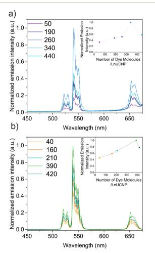
**Fig. 2** (a) Upconversion emission spectra of the SL system with different numbers of dye molecules per LnUCNP. (b) Upconversion emission spectra of the SE system with different numbers of dye molecules embedded into the silica sell per LnUCNP.
