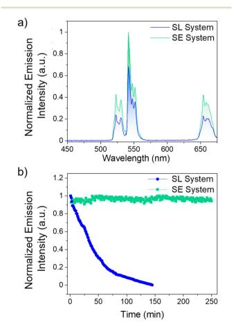
Fig. 3 (a) Normalized upconversion emission spectra of the SL and SE systems under 800 nm excitation. (b) Emission intensity of the  $^4\text{S}_{3/2}$ ,  $^2\text{H}_{11/2} \rightarrow ^4\text{I}_{15/2}$  transition of Er<sup>3+</sup> in the SL (blue) and SE (green) systems as a function of time under 800 nm excitation.
