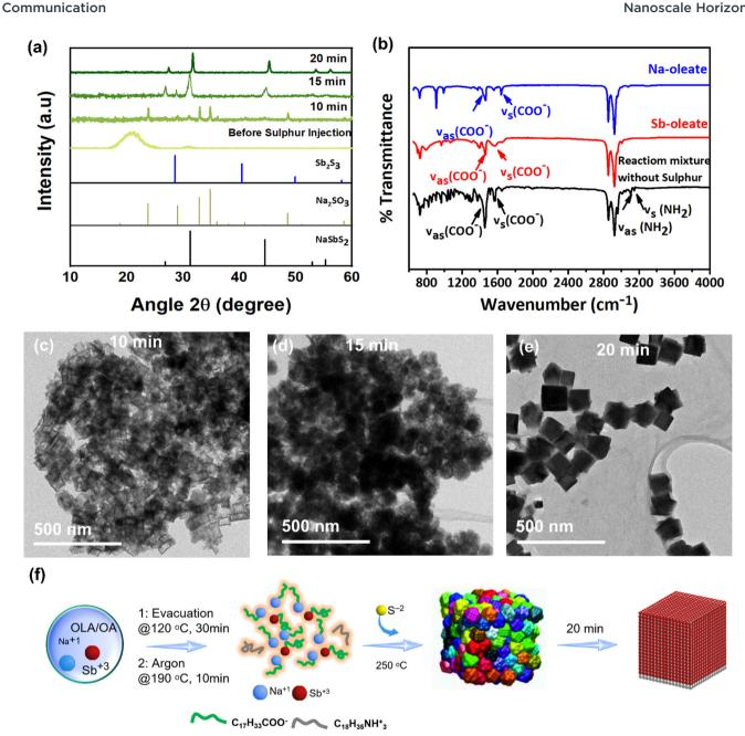
Fig. 5 (a) XRD spectra showing the phase evolution of NaSbS<sub>2</sub> NCs at different reaction time i.e. before injection of sulphur and after injection of sulphur precursor (10, 15 and 20 min) along with (b) FTIR spectra of aliquot taken before injection of sulphur. Panels (c and e) show the TEM images for 10, 15 and 20 min respectively. (f) Schematic depiction of time lapsed phase evolution of NCs.
