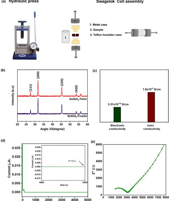
Fig. 6 (a) Schematic for Swagelok cell assembling (b) XRD pattern of the pellet and powder NaSbS<sub>2</sub> before and after cold press (c) bar graph of electronic and ionic conductivity (d) DC polarization of NaSbS2 with inset showing the current behaviour for duration of 5000 s (e) Nyquist plot of Electrochemical Impedance Spectroscopy (EIS) of NaSbS<sub>2</sub> pellet.
