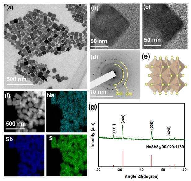
Fig. 1 TEM image (a) of NaSbS<sub>2</sub> NCs with (b and c) tilted TEM imaged at an angle of  $\pm 30^{\circ}$  with (d) SAED and (e) crystal structure showing mixed cation sites of NaSbS2 yellow (S), red (Na) and blue (Sb). (f) EDX elemental mapping for distribution of the three elements and (g) XRD pattern showing match to cubic phase NaSbS<sub>2</sub> (00-029-1169).
