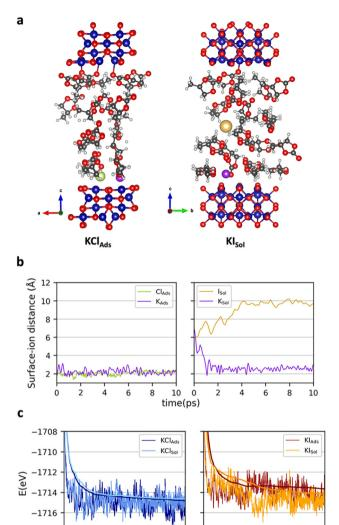
Fig. 2 (a) Representative snapshots of the most favorable KCl<sub>Ads</sub> and KI<sub>Sol</sub> AIMD simulations; variation along the AIMD simulation of the (b) surfaceion distance (K, Cl and I) at the most favorable conformation and (c) energy. Label code: Co (blue), O (red), C (black), H (white), K (purple), Cl (green), I (pale orange).
