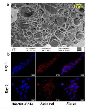
Fig. 1 (a) The SEM image of a CA scaffold showing an average pore size  $50~\mu m$ . (b) Confocal image of the NIH 3T3 cells grown on the CA scaffold on day 3 and day 7. Cell nuclei are stained with Hoechst 33342, and the cytoskeleton is stained with actin red. All the images are captured at a magnification of  $63\times$ .
