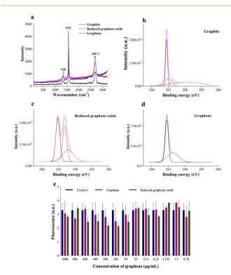
Fig. 3 (a) Raman spectra of graphite, reduced graphene oxide, and graphene. X-ray photoelectron spectrograph of (b) graphite, (c) reduced graphene oxide, and (d) graphene, and (e) toxicity assay for graphene and reduced graphene oxide.
