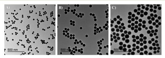
Fig. 2 TEM images and size distribution of core-shell nanosystems (A) DC 50 (49  $\pm$  3 nm), (B) DC 90 (93  $\pm$  4 nm) and (C) DC 120 (116  $\pm$  3 nm).
