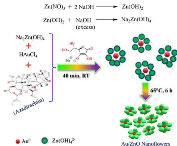
**Scheme 6** Schematic chart of the fabrication procedure of Au/ZnO hybrid nanoflowers using *A. indica* (neem) leaf extract. Reprinted with permission from ref. 79. Copyright © 2021, American Chemical Society.
