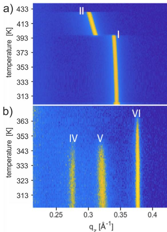
**Fig. 4** Temperature-dependent *in situ* XRD measurements for OEG-BTBT films, prepared *via* drop casting, in a waterfall plot. (a) Thin film of Form I prepared from chloroform solution, and (b) thin film containing all three new solvates simultaneously.
