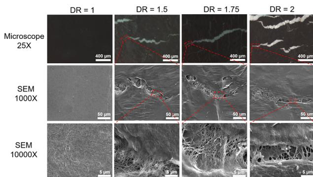
Fig. 4 Optical microscope and SEM images of heat-repaired CNT veils after stretching at different draw ratios DR. The scale bars are  $400 \mu\text{m}$ ,  $50 \mu\text{m}$  and  $5 \mu\text{m}$ , respectively, from top to bottom row.
