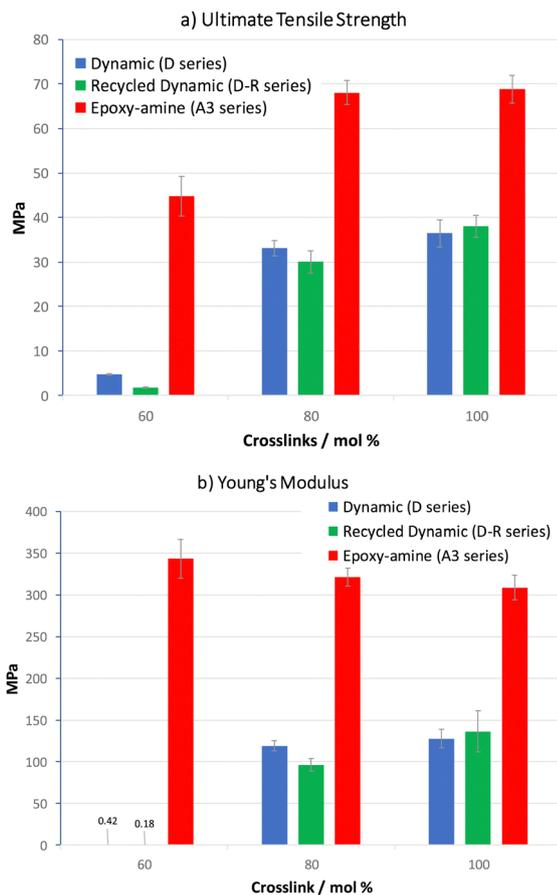
Fig. 11 (a) Ultimate tensile strength and (b) Young's modulus, data for D60–D100 and A<sup>3</sup>60–A<sup>3</sup>100 materials.
