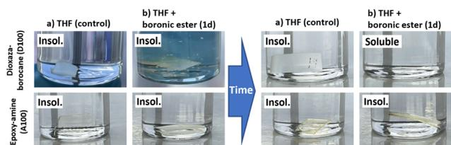
Fig. 9 Chemical recycling of D100, using *n*-butyl phenylboronic ester **1d**. (a) immersion of epoxy-amine-dioxazaborocane D100 and epoxy-amine A100 in THF at the start of the experiment and after 24 hours. (b) shows immersion of D100 and A100 in THF with *n*-butyl phenylboronic ester **1d** at the start of the experiment and after 24 hours.
