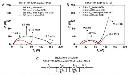
Fig. 5 EIS at the half-wave potential ( $E_{1/2} = 3.66 \text{ V}$ ) for 50 wt% PTMA-GMA on (A) rGO/BANF and (B) Al foil before and after rate capability testing. (C) Fitted equivalent circuit for 50 wt% PTMA-GMA on rGO/BANF and Al foil.
