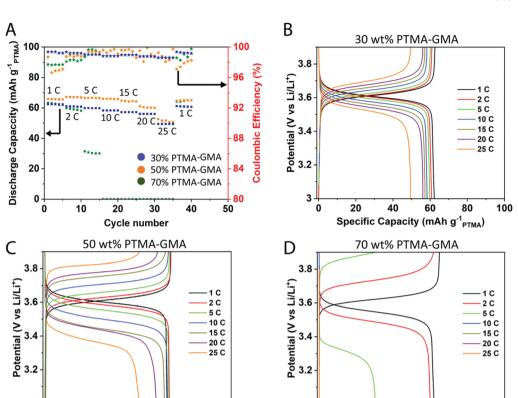
Fig. 2 (A) GCD testing showing different C-rates for 30 wt% PTMA-GMA, 50 wt% PTMA-GMA, and 70 wt% PTMA-GMA electrodes on rGO/BANF. GCD curves at different C-rates for (B) 30 wt% PTMA-GMA, (C) 50 wt% PTMA-GMA, (D) 70 wt% PTMA-GMA electrodes on rGO/BANF. The cell configuration was a lithium metal half-cell, and the electrolyte was 1 M LiPF<sub>6</sub> in EC/DEC (1:1 v/v) as the electrolyte. Specific capacities are reported based on the PTMA-GMA mass loading
