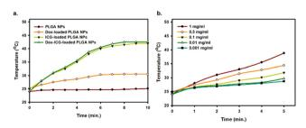
Fig. 4 Comparison of the photothermal conversion efficiency of the synthesized NPs in different formulations. (a) The temperature elevation curves of blank PLGA NPs, Dox-loaded PLGA NPs, ICG-loaded PLGA NPs, and Dox-ICG-loaded PLGA NPs in response to 5 min NIR irradiation (808 nm laser, 2 W cm<sup>-2</sup>). (b) The concentration-dependent thermal heat generated curve of Dox-ICG-loaded PLGA NPs as a function of NIR irradiation time
