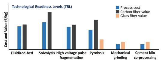
Fig. 10 Relative costs and values of resin composite recycling technologies (the sizes of the bars are indicative and vary among EU recyclers using the same process due to varying process parameters such as throughput rates/capacity, temperature/pressure and retention time in the reactor). 14
