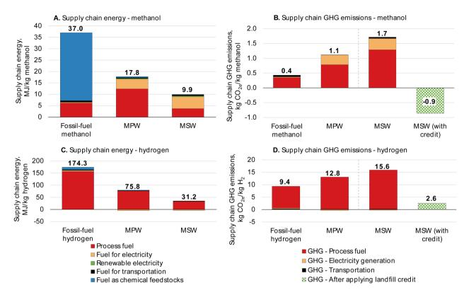
Fig. 7 Materials Flows through Industry supply chain results for the process configurations presented for all four cases in this analysis. Supply chain energy requirements decrease for MPW- and MSW-based processes because feedstock is considered "waste" without any inherent energy. GHG emissions for all MPW cases increase from fossil-fuel counterparts. The credit for MSW is due to the avoidance of CO2 emissions at the landfill. All results from the MFI analysis are given in Tables S18 and 19.†
