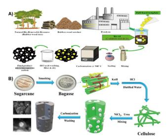
Fig. 19 (A) Schematic designs of resource collection and synthesis route of hierarchical porous hard carbon. 197 Reprinted with permission. Copyright 2019, Elsevier. (B) Flow chart of as-synthesized biomass porous carbon materials.<sup>201</sup> Reprinted with permission. Copyright 2021, Elsevier.
