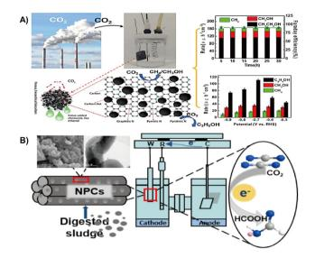
**Fig. 12** (A) Municipal sludge derived carbon dots modified, N-doped biochar for the electrochemical reduction of carbon dioxide. Reprinted with permission. Copyright 2022, Elsevier. (B) Nitrogen-doped porous carbon from digested sludge for the electrochemical reduction of carbon dioxide to formate. Reprinted with permission. Copyright 2018, American Chemical Society.
