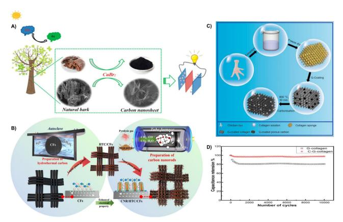
Fig. 22 (A) Preparation of the 3D porous carbon nanosheet.<sup>220</sup> Reprinted with permission. Copyright 2019, American Chemical Society. (B) The schematic diagram of the synthesis of CNR/HTC/CFs. 219 Reprinted with permission. Copyright 2021, Elsevier. (C) Schematic demonstration of collagen, G-collagen, and C-G-collagen fabrication. (D) Cyclic study of C-G-collagen.<sup>223</sup> Reprinted with permission. Copyright 2022, Elsevier.
