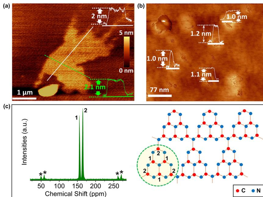
**Fig. 2** (a) AFM image of g-CN nanosheet with sectional profile measurement showing height and thickness profiles (nm). (b) AFM images of nanosheets with respective height profiles at different locations. (c) Solid-state  $^{13}\text{C}$  NMR spectra of as-prepared g-CN and its idealized structure showing heptazine tectonic units.
