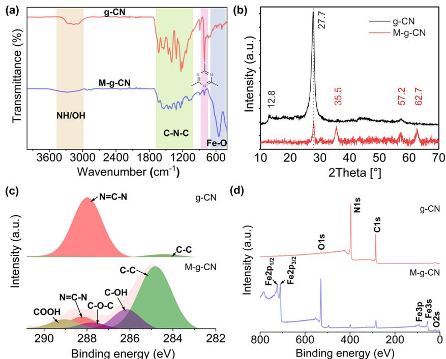
**Fig. 1** Crystalline and phase studies of as-synthesized g-CN and M-g-CN (a) FT-IR spectra showing different functionalities of the samples with distinct characteristics. (b) XRD pattern of samples. (c) High-resolution C1s spectra. (d) Survey profile with an arrangement of elements.
