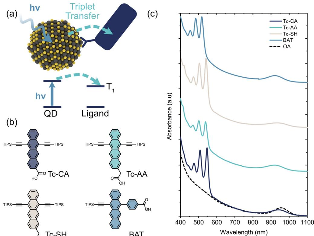
**Fig. 1** (a) Schematic illustration of the triplet sensitization process studied herein. A quantum dot (QD) absorbs a photon whereupon the exciton is transferred to an energetically available triplet state on a surface-anchored organic ligand. (b) Molecular structures of the four tetracene based ligands used as triplet acceptors. (c) Absorption spectra of the PbS/ligand QDs used in this study, compared to the as synthesized oleic acid (OA)-capped PbS QDs.
