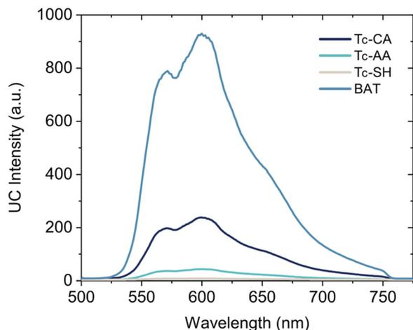
Fig. 4 Upconverted anti-Stokes emission upon 785 nm excitation of samples containing PbS/Ligand and 10 mM Rubrene in oxygen free toluene. Laser scatter is filtered by a 750 nm short pass filter.
