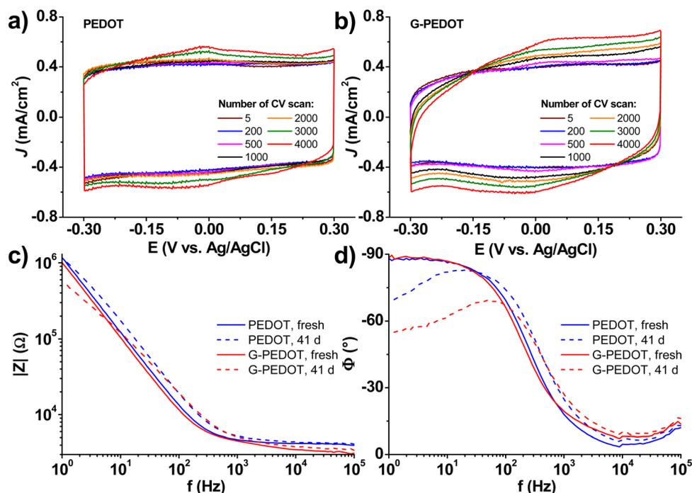
**Fig. 4** Electrochemistry of PEDOT and G-PEDOT microelectrodes (50 × 50 μm) prepared by galvanostatic electropolymerization (2 μC: 20 nA, 100 s) (a and b): selected cyclic voltammograms (scan rate = 100 mV s<sup>-1</sup>) over 4000 cycles (electrochemical stability test); (c and d): electrochemical impedance spectra (bode plots, averaged over 2–3 different specimens) as prepared and after 41 days of accelerated aging test (60 °C, PBS solution).
