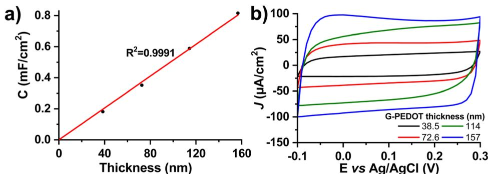
**Fig. 3** Electrochemical capacitance of G-PEDOT. (a) Linear dependence of areal capacitance on the layer thickness. (b) Cyclic voltammograms (0.1 M KCl,  $100 \text{ mV s}^{-1}$ ) used for calculation of the capacitance.
