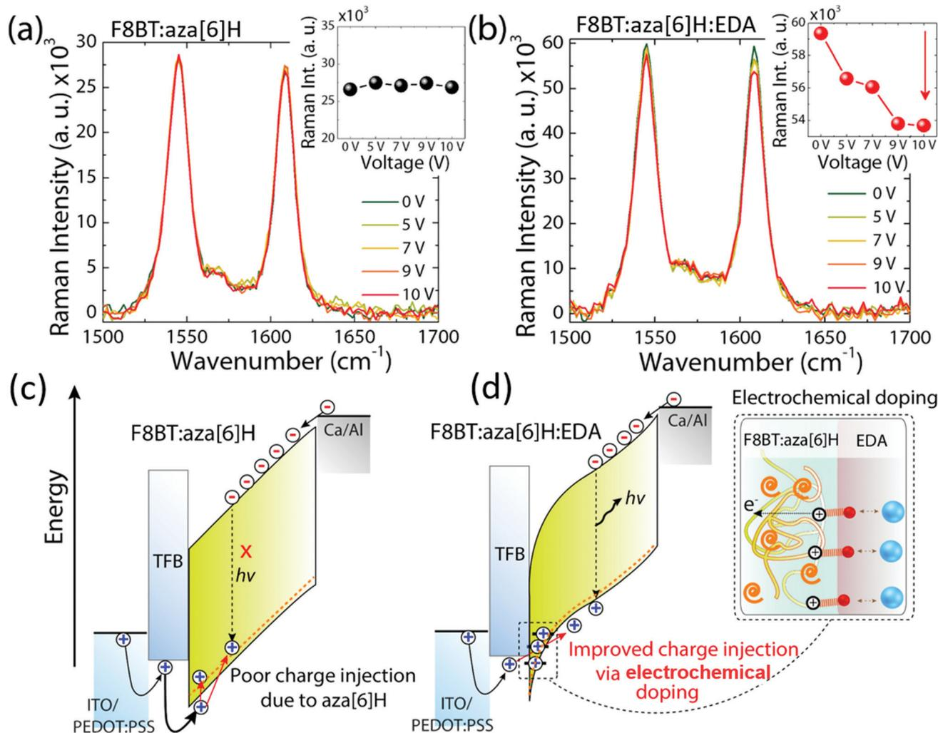
Fig. 5 (a) and (b) *In situ* electric-field-dependent Raman spectra of the F8BT:aza[6]H and F8BT:aza[6]H:EDA devices, respectively. The inset figures indicate the changes in the selective Raman peaks at 1608  $\text{cm}^{-1}$  under an electric field ranging from 0 V to 10 V. (c) and (d) The proposed mechanism of poor charge injection in F8BT:aza[6]H and improved charge injection and charge balance in an EDA-doped device via the electrochemical doping by EDA molecules (inset), respectively.
