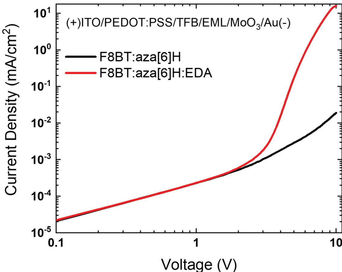
Fig. 4 (a)  $J$ - $V$  characteristics of the F8BT:aza[6]H and F8BT:aza[6]H:EDA hole-only devices (ITO/PEDOT:PSS/TFB/EML/MoO<sub>3</sub>/Au).
