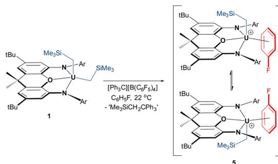
Scheme 3 Synthesis of fluorobenzene-coordinated uranium alkyl cation  $5$  ( $\text{Ar} = 2,6$ -diisopropylphenyl), which in solution, on the NMR timescale, undergoes rapid migration of the alkyl group from one side of the plane of the ligand backbone to the other.
